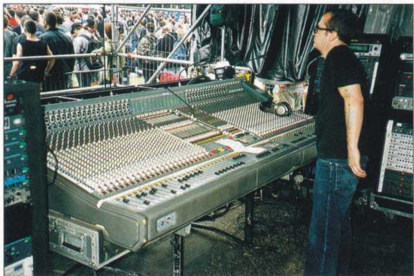
The Adamson system was controlled by a Midas desk FOH
