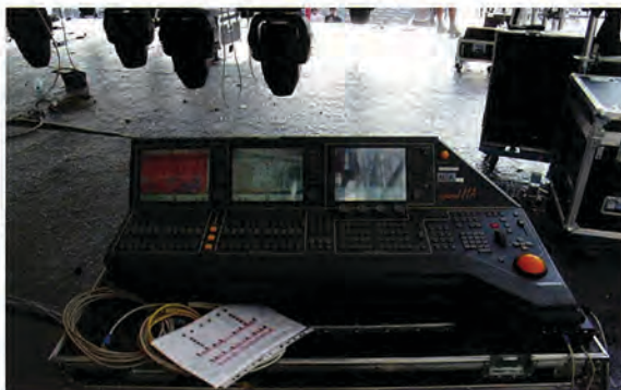
A GrandMa lighting desk is outfitted with a new RDMX08AC cable to the dimmers
