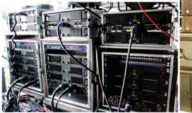
Lab.gruppen amplifiers and XTA DSP processors located under the stage 1 right area to serve the right hand speaker system
