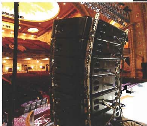
A groundstacked Adamson Y10 array, the most frequent method of deployment on the tour.
